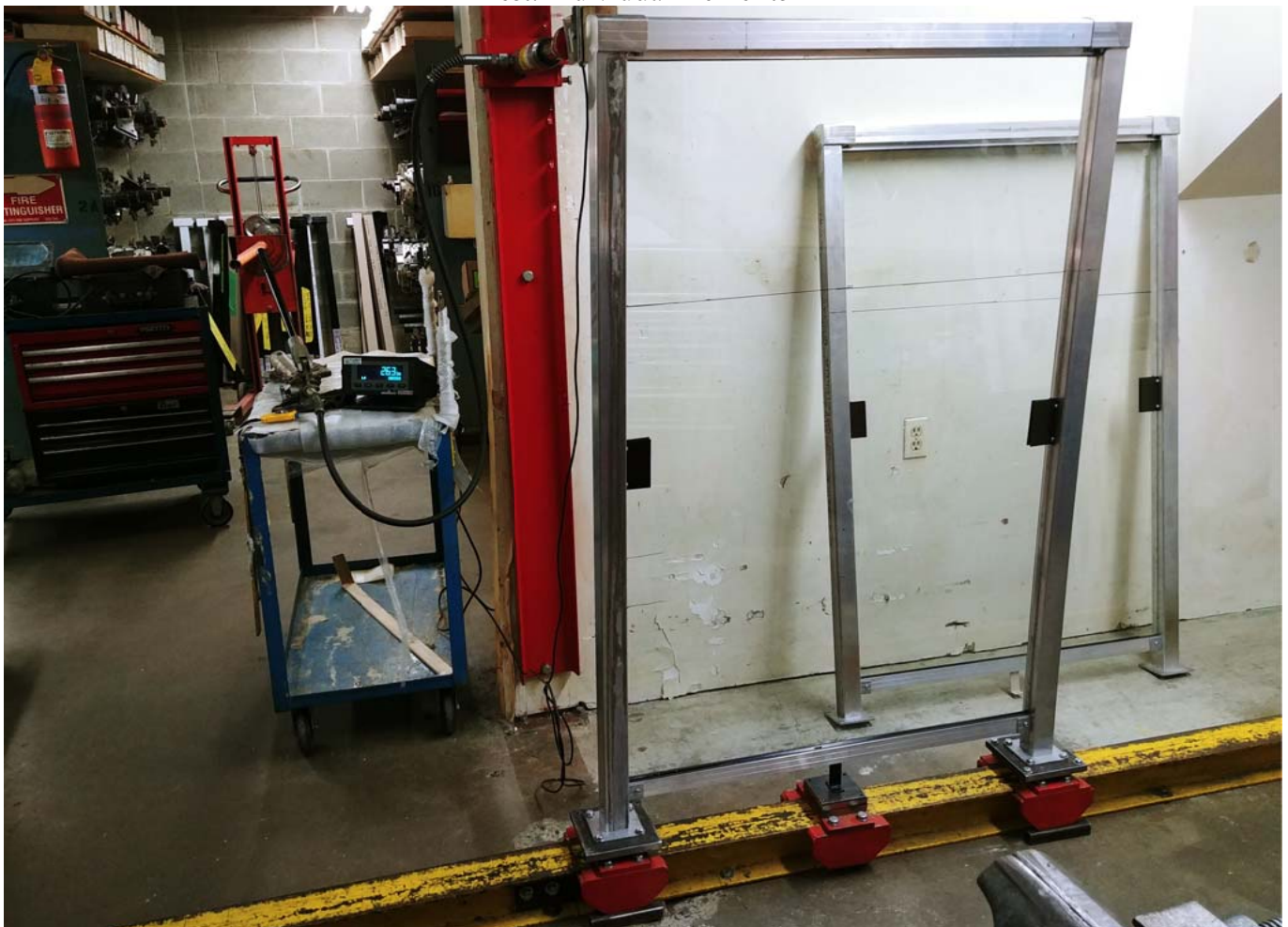
Test: Top Of Post Concentrated Load
