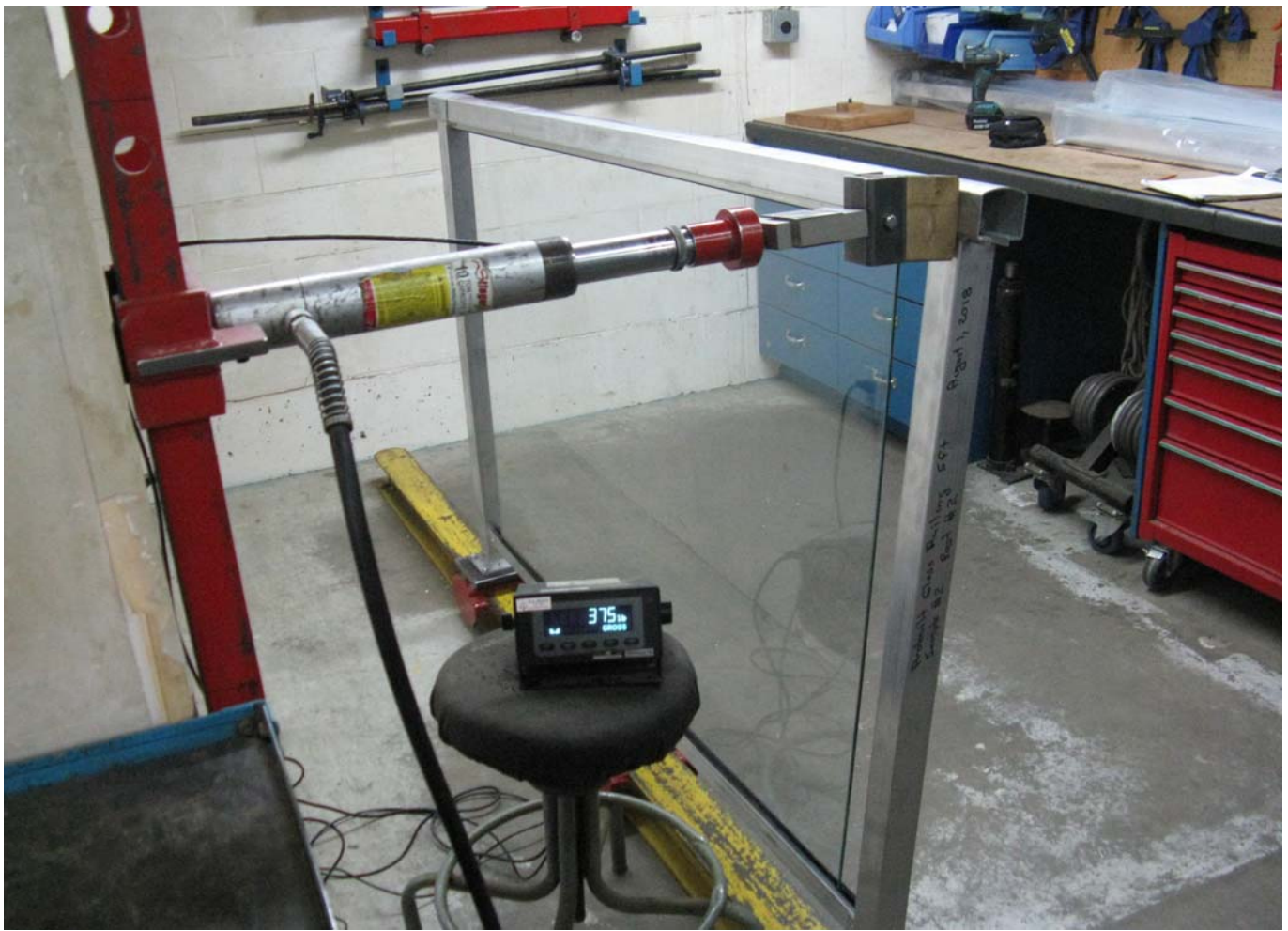
Test: Top Of Post Concentrated Load
